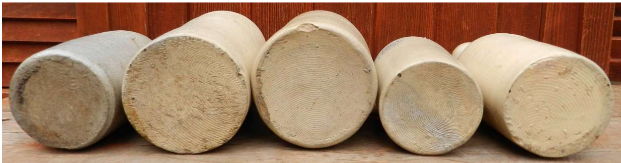
Figure 3 The bottoms of these bottoms have lines that are the result of cutting the bottle with a wire to remove it from the wheel. In the 1860's potters often used a pair of wires twisted together which created these lines. In later years potters used a single wire that resulted in a smooth bottom.
